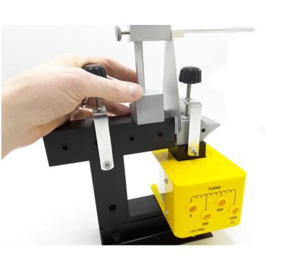
5) Turn on the power supply an swing the slotted pendulum. Does the pendulum slow down appreciably as it passes through the gap?
