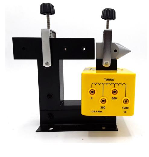
4) Mount the pendulum with the slots in it as shown in the picture below. The top of the slots should be just above the top of the I-core.
